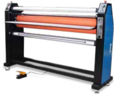
The Paramount 65X is the Pneumatic Laminator you have been waiting for. Backed by over 30 years of industry experience, the 65" pneumatic pressurized rollers offer trouble free lamination. With maximum speeds reaching nearly 20 ft./min. (6 m./min.) and the included rear take-up, the Paramount 65X sets a new standard for wide format laminators.
