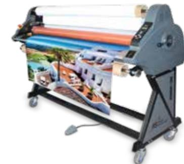
Royal Sovereign laminators with the unique heat assist top lamination roller helps activate the adhesive of pressure sensitive laminates for a smooth clear finish and shorter laminate cure times. The added heat helps reduce the phenomenon known as "silvering" when using some cold lamination films.
